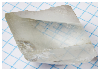
Figure 2: Double refraction of a calcite crystal. The two images of a blue line come from the two orthogonal polarities which are refracted by a different angle. Image by APN MJM [APN11].
